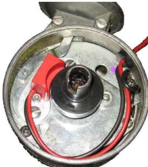
Example of a Hot-Spark kit in a Ford vacuum-advance distributor
