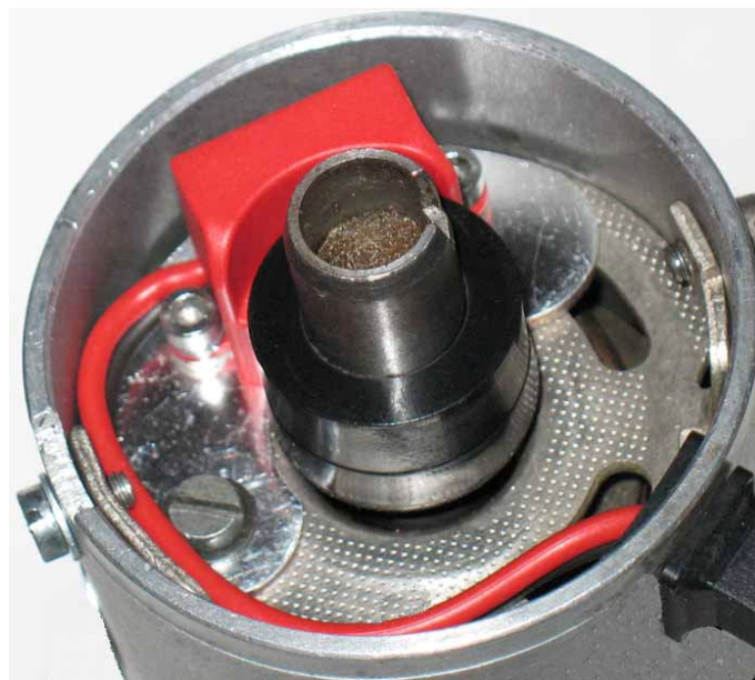
Example of Hot-Spark kit in a Bosch 009 non-vacuum-advance distributor
